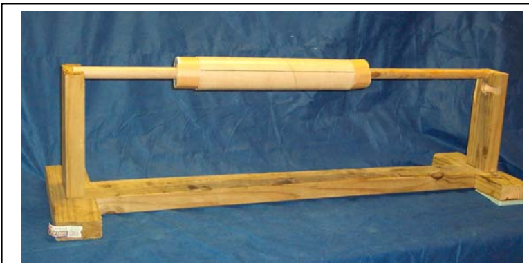
Photo 1 – Airframe tube on turning jig. (photo taken by Bart Merkley)
