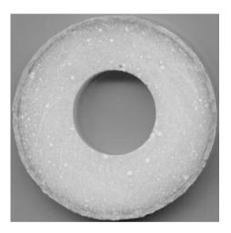
**Cut through propellant segment**
