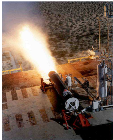
Figure II-1: The 250,000 lb thrust motor, utilizing LOX and HTPB
