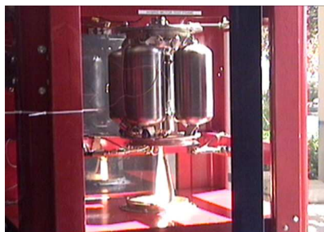
Figure II-2: MoTV-1 Prototype MoTV using N 2 O / PMMA
