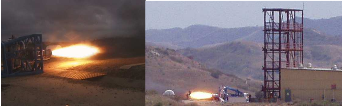
Figure II-4 Test Firing of Streaker SLV Hybrid Upper Stage Using Nitrous Oxide and HTPB
