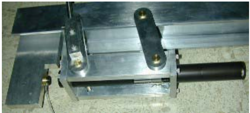
Figure 5 is a photo of our motor sitting in a test stand. The load cell stand will be mounted to a concrete and wood base that is under construction on a secluded 20-acre plot south of Indianapolis. Although the test stand will accommodate motors up to 2,200 pounds thrust, our wax hybrid falls into the "J" class.
