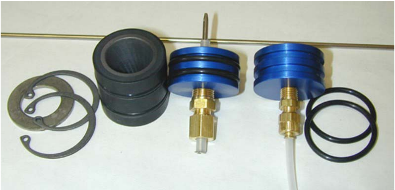
Figure 2 is a photo of the actual components of the hybrid test motor. The parts are anodized to provide a burn-resistant surface.
