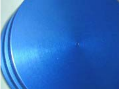
Figure 4 is a photo of the vent hole in the forward bulkhead. It is .009" diameter and vents through a 1/8" diameter nylon tube to a port on the rocket body tube.
