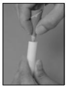
**9.** Label each motor with a serial number. Record serial numbers and any noteworthy aspects of motor assembly in a notebook. Let the nozzle dry for 24 hours. Then **make sure the narrowest part of the nozzle is at least 9/64**" in diameter by checking with the drill bit.. Mix the propellant:
