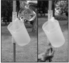
water at a time, until the container reaches the bottom of the test stand. Each mark represents two Newtons. The peak thrust could be as high as 16 Newtons (about 3.5 pounds). Make sure your stand can handle that.
