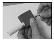
**8.** Cut the sandpaper into four pieces. Forming a piece into a cone which diverges at a  $15^{\circ}$  angle. Turn the sandpaper cone by hand to widen the aft (exposed) end of the nozzle so that the bottom half of the nozzle diverges at a  $15^{\circ}$  angle.
