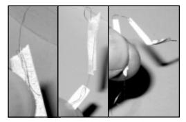
motor), to make sure the wire burns quickly, and **only at the single strand portion** in its center.
